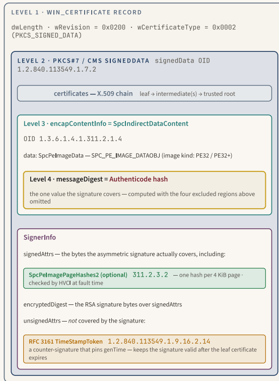
Read top-down: the optional header points by file offset at the WIN_CERTIFICATE, which wraps SignedData, whose SpcIndirectDataContent carries the one signed value — the Authenticode hash. The certificate table is itself excluded, so the signature can live inside the very bytes its hash omits.
