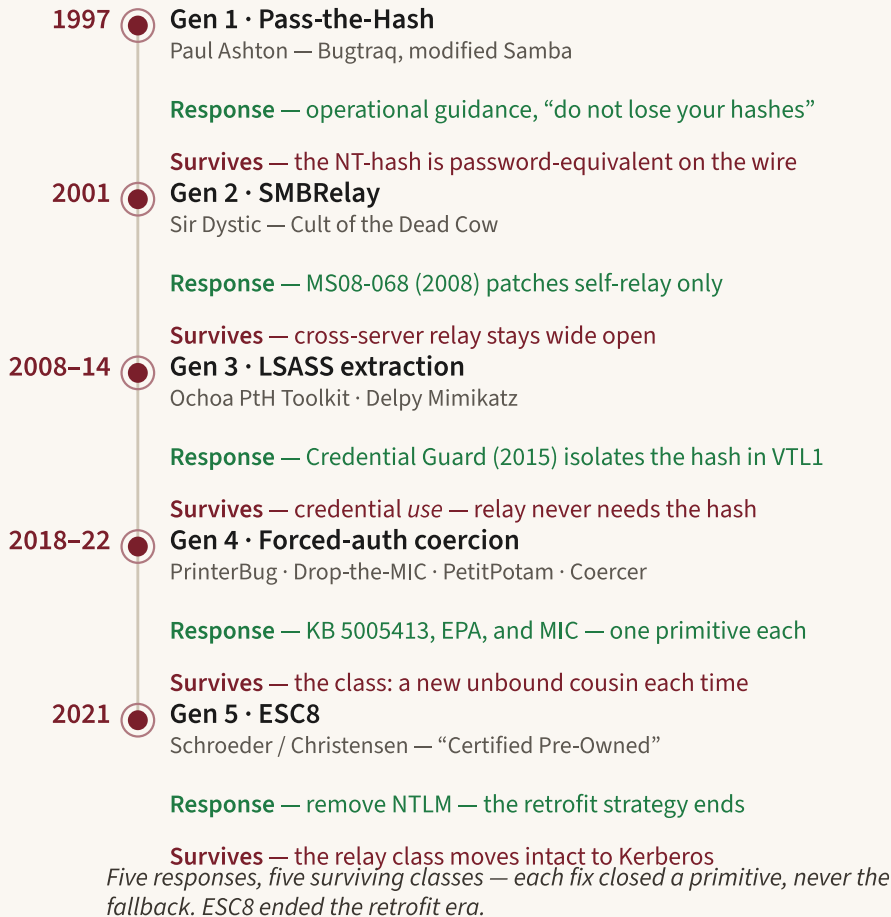
Figure 16.3: Five generations of NTLM attacks, 1997–2021, as a dated timeline. Each generation pairs the named attack with the Microsoft response and the class that response left alive: Pass-the-Hash (operational guidance; the hash stays password-equivalent), SMBRelay (MS08-068 patches self-relay only; cross-server relay survives), LSASS extraction (Credential Guard isolates the hash; credential use survives), forced-auth coercion (KB 5005413, EPA, and MIC per primitive; the class survives), and ESC8 (remove NTLM; the relay class moves intact to Kerberos). The cadence is the argument. Every fix closed a primitive, never the fallback, until ESC8 ended the retrofit strategy.
